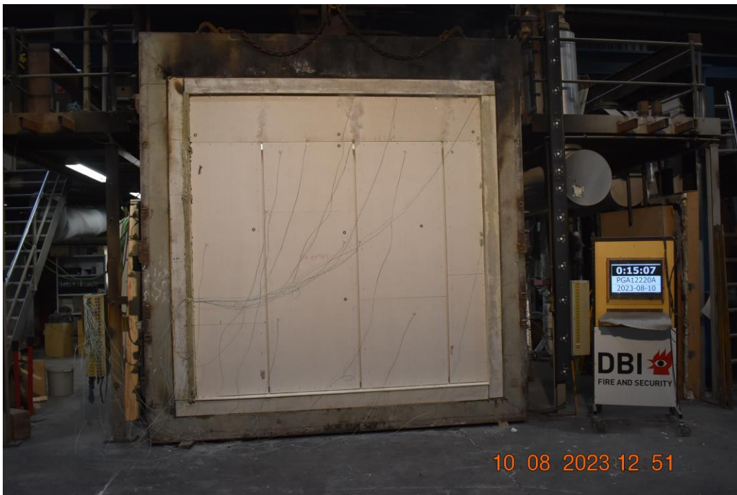
Photo No. 12 Test specimen after 15 minutes of testing.
