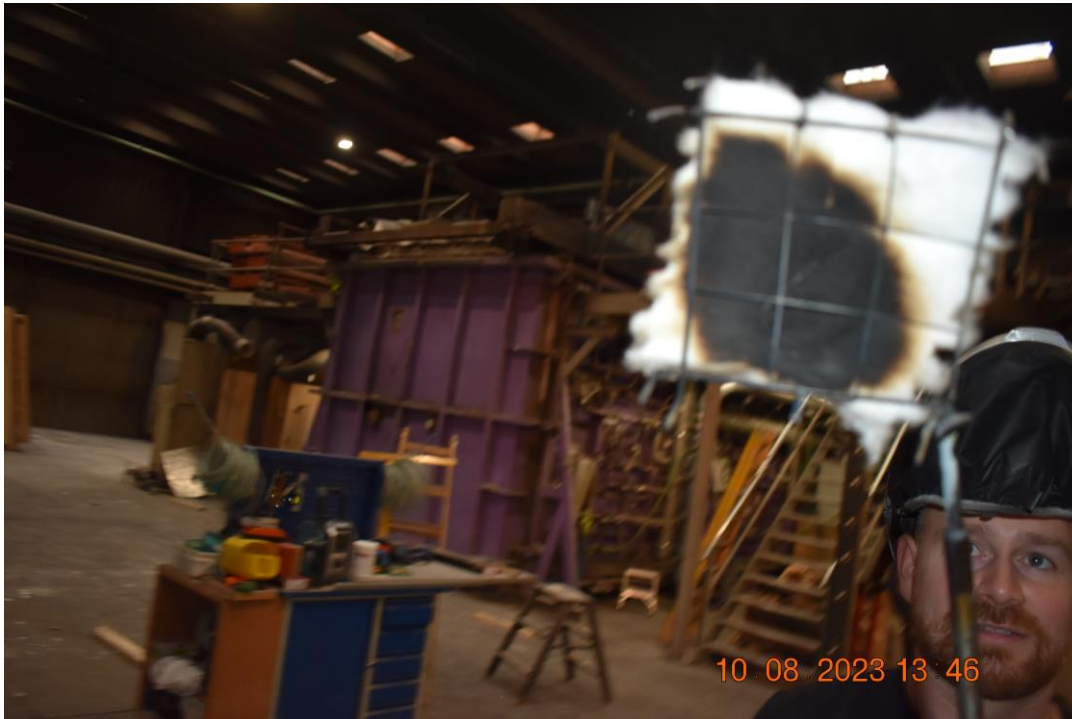
Photo No. 23 Heavy charring but no flame or embers. Eight cotton pad test.
