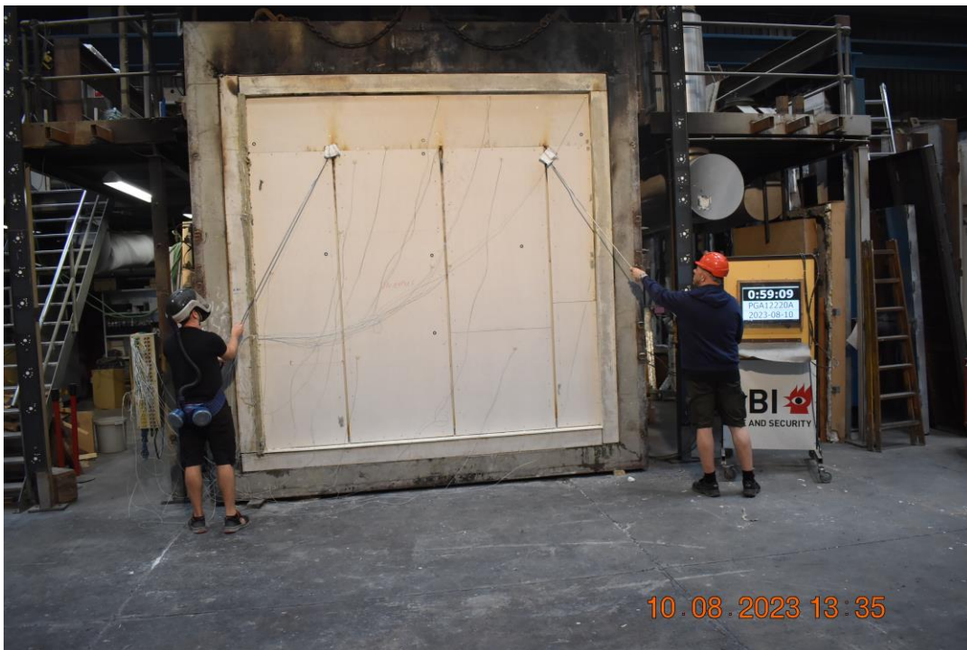
Photo No. 16 Test specimen after 59 minutes of testing. Fourth and fifth cotton pad test.
