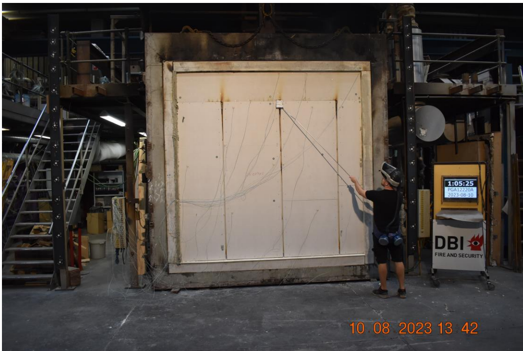
Photo No. 18 Test specimen after 65 minutes of testing. Sixth cotton pad test.
