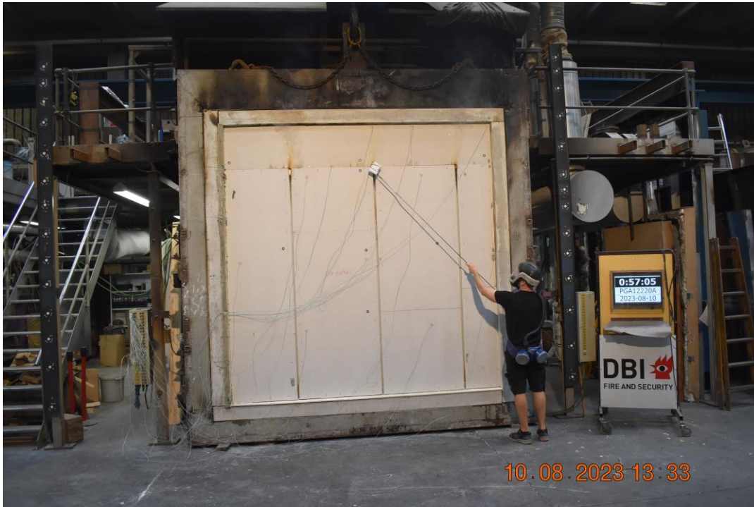
Photo No. 15 Test specimen after 57 minutes of testing. Third cotton pad test.
