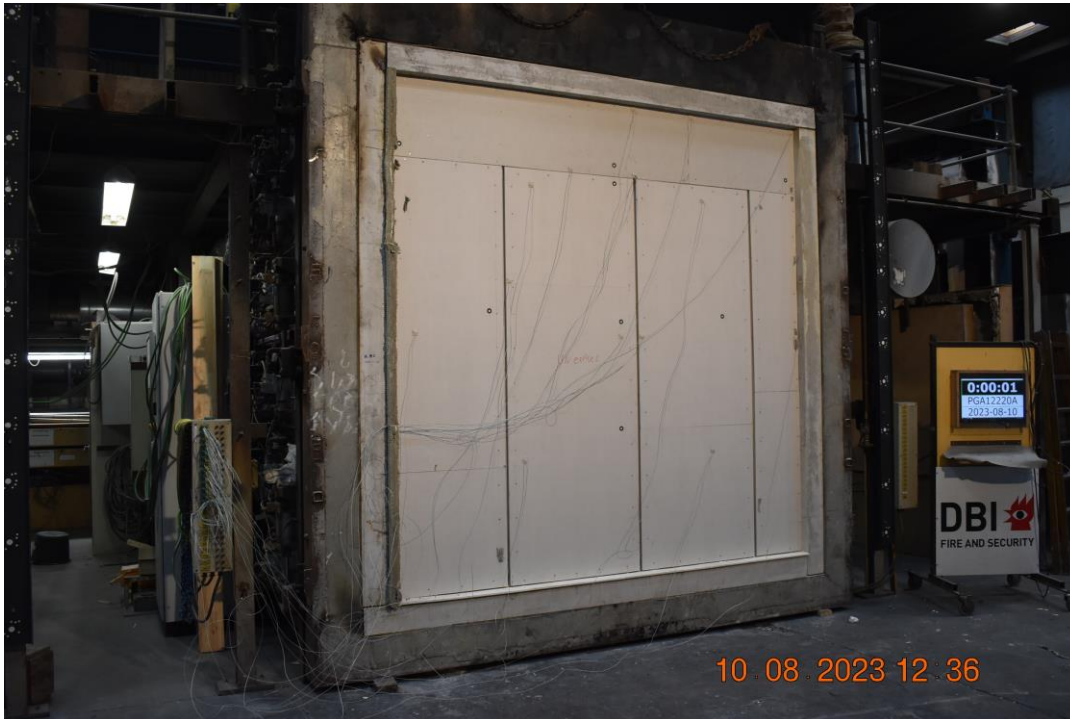
Photo No. 11 Test specimen at beginning of test.
