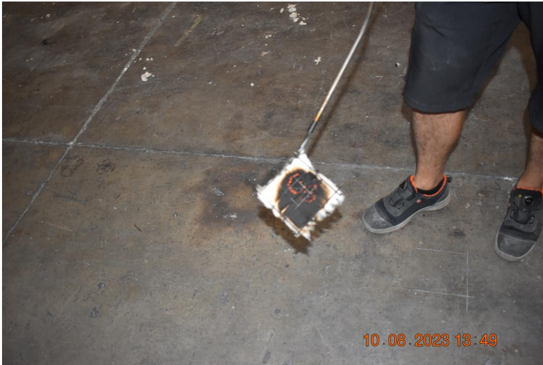
Photo No. 27 Heavy charring and embers. Tenth cotton pad test.
