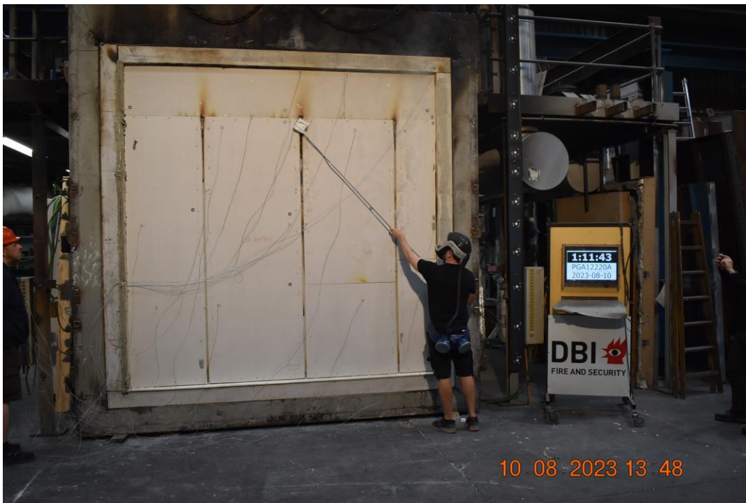
Photo No. 26 Test specimen after 71 minutes of testing. Tenth cotton pad test.
