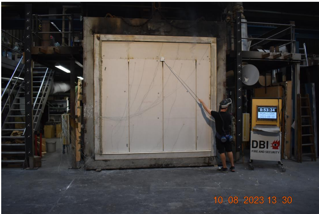
Photo No. 14 Test specimen after 53 minutes of testing. Second cotton pad test.
