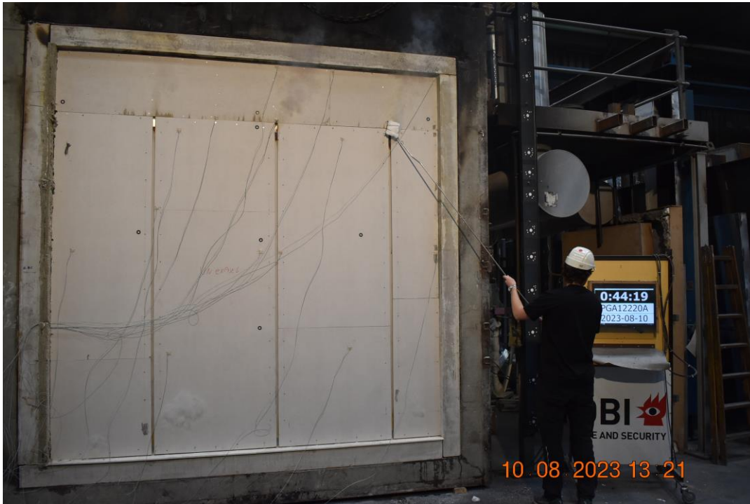
Photo No. 13 Test specimen after 44 minutes of testing. First cotton pad test.
