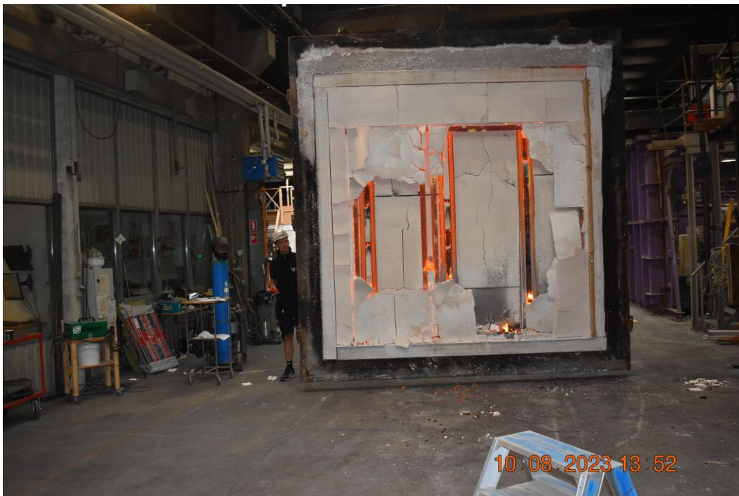
Photo No. 28 Test specimen after removed from furnace, seen from exposed side.
